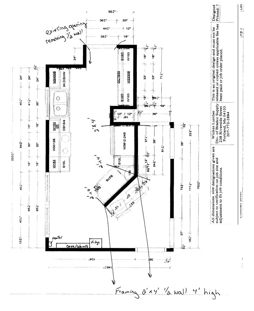
Relocate bathroom fixtures & remove non-bearing wells.
