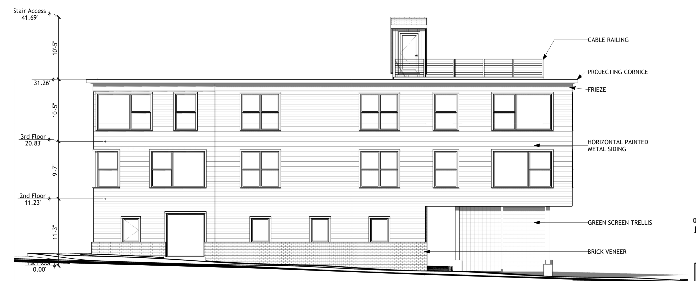
4 : South Elevation : 1/8 in = 1 ft
