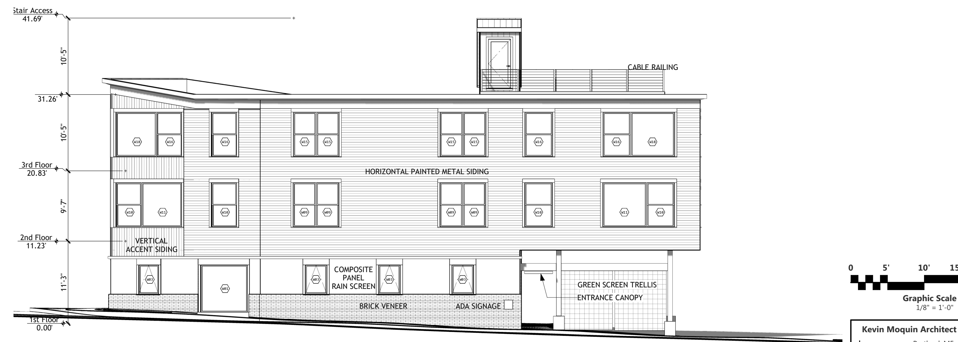
4 : South Elevation : 1/8 in = 1 ft
