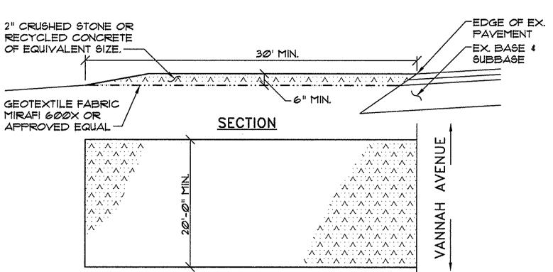
I. ENTRANCE TO BE PLACED WHEN PAVEMENT IS REMOVED. WHILE EXISTING PAYEMENT REMAINS THE ENTRANCE IS NOT REQUIRED.
