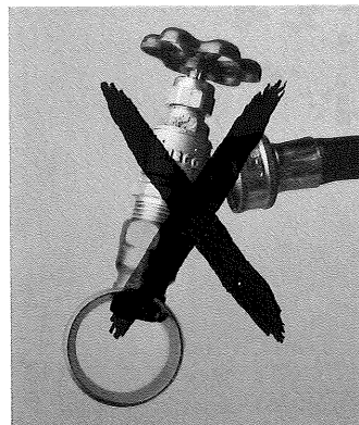
"Turned tees" in water lines restrict flow, create turbulence and bending stress on hoses.
