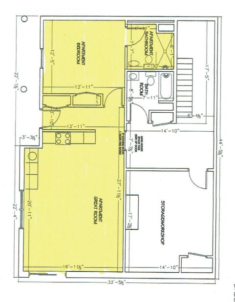
GROSS BASEMENT AREA 1,408 SF APARTMENT AREA 717 SF OR 25% ALLOWABLE BASEMENT AREA 704 SF TOTAL ALLOWABLE AREA (MAIN FLOOR + 704 SF) 2,812 SF
