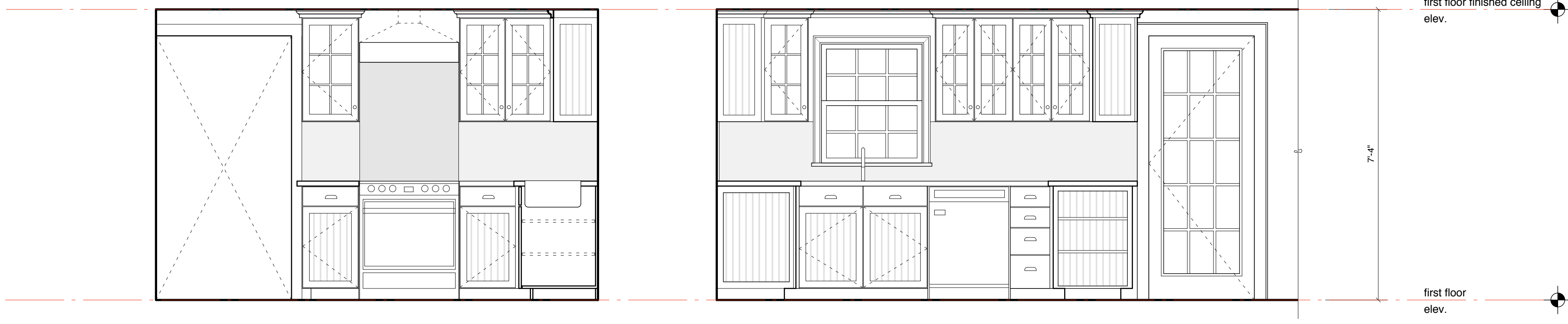
7A North Elevation-Option A-no demolition of existing exterior west wall SCALE: 1/2" = 1'-0" GLASS DOORS ON UPPER CABINETS
