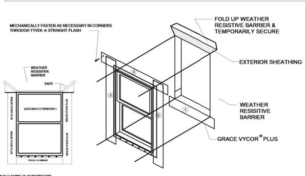
ASHING TIE-IN INSTRUCTIONS: FOLD UP & TEMPORARILY SECURE WEATHER RESISTIVE BARRIER LASHING UNDER WEATHER E BARRIER BACK OVER HEAD FLASHING AND
