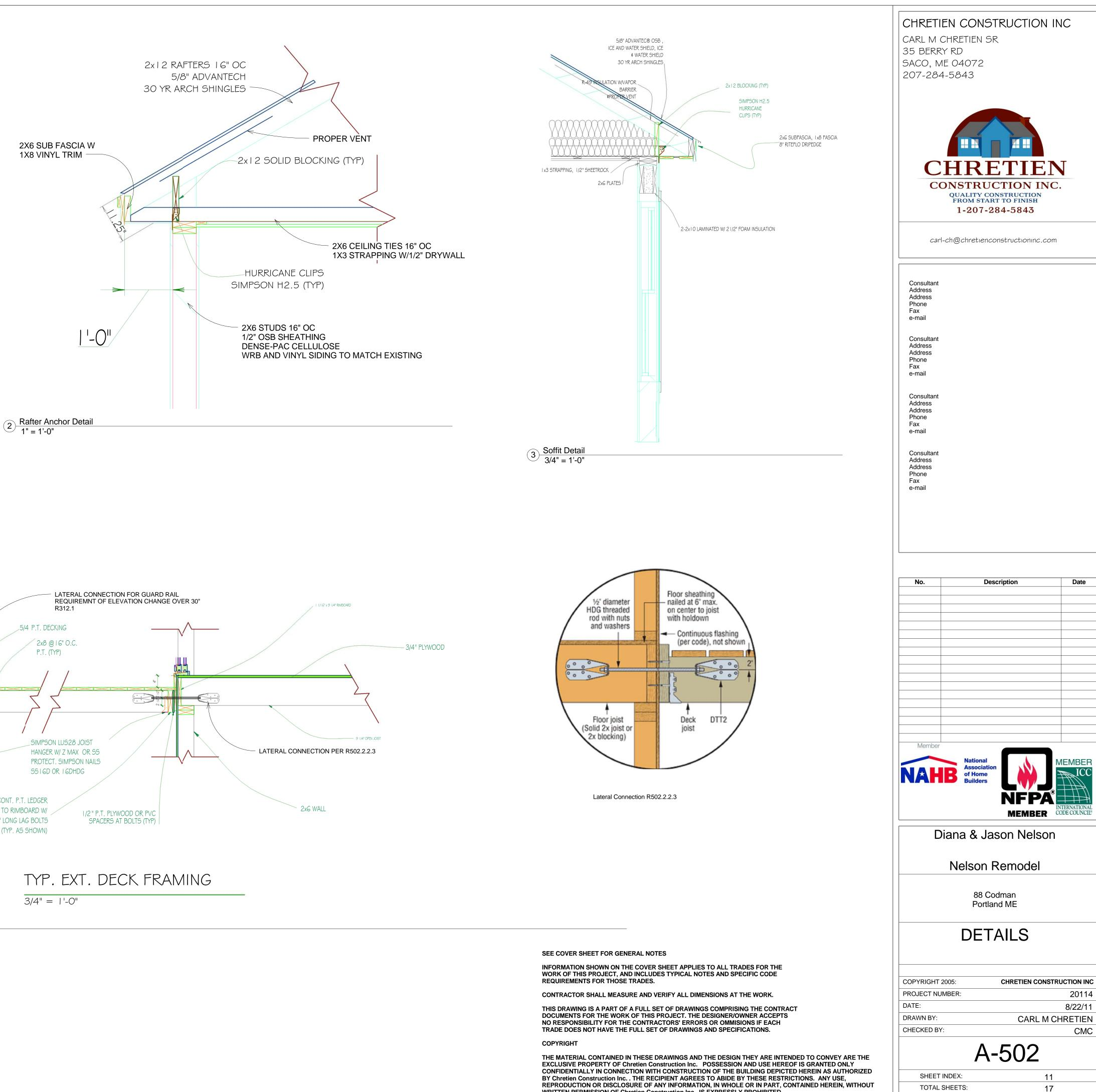
2x8 CONT. P.T. LEDGER FASTEN TO RIMBOARD W/ 5/8" Ø x 5" LONG LAG BOLTS @ 6" O.C. (TYP. AS SHOWN)
