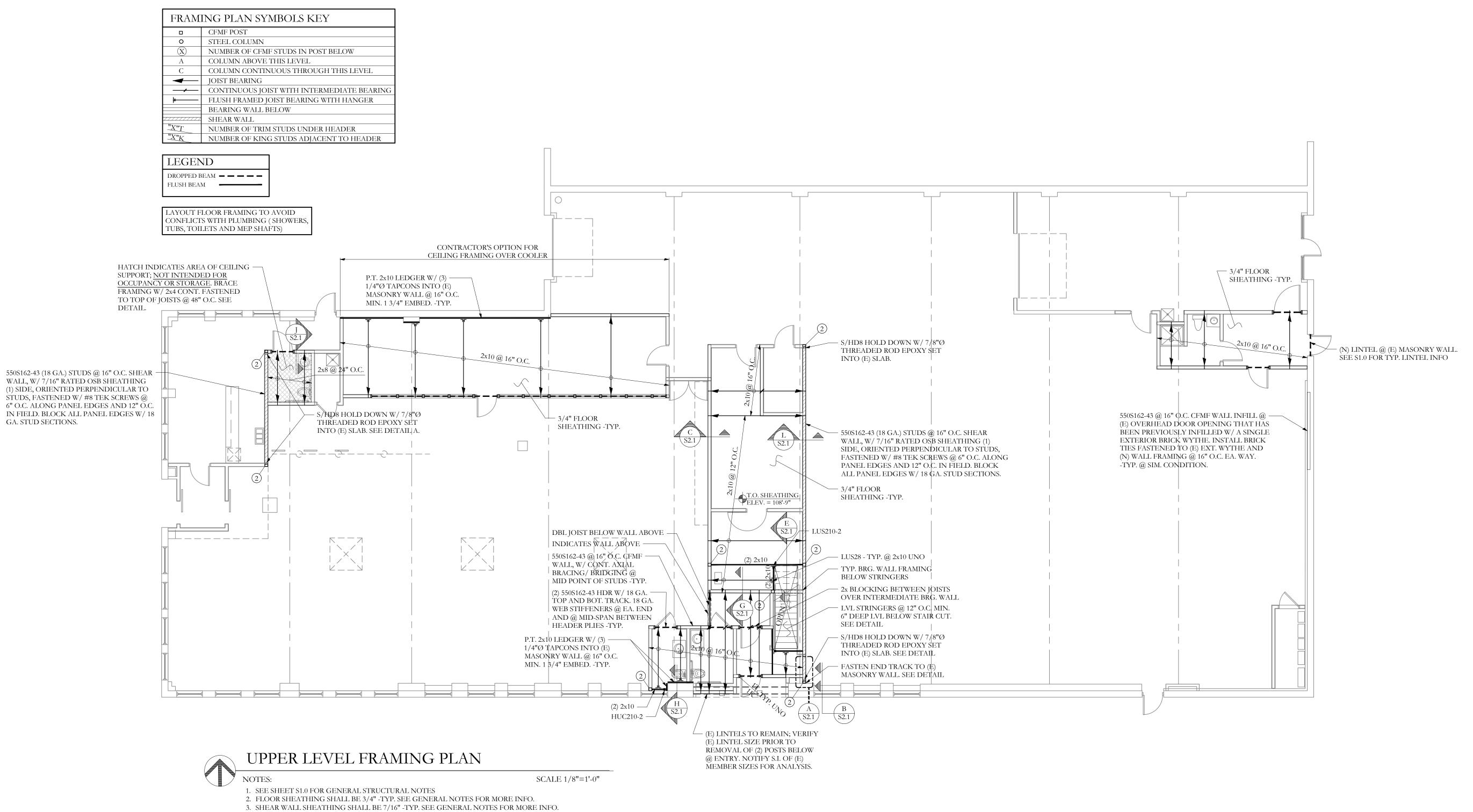
4. USE MIN. #10 SCREWS AT ALL CFMF CONNECTIONS -TYP. UNO
