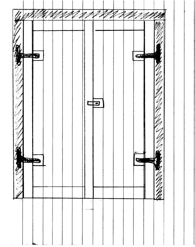
DOOR (45" opening) (2) =" PLYWOOD PANEUS 33 /21 \* 4" FRAME AROUND PANELS 1" OUBRUAP (1x4) ON SHORTER PAner Spring Combad Hinges (2) Supra Locks on TOP/BOTTOM OF SMAUGR DOOR. Locking HASP Wood GLUE AND 12" SCREWS FOR PANEL CONSTRUCTION 2" NAILS FOR OUTSIDE FRAME
