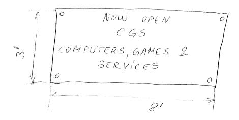
will be attached to Blog with 4 HEAVY DUTY WAShers and Screws 3 inch long
