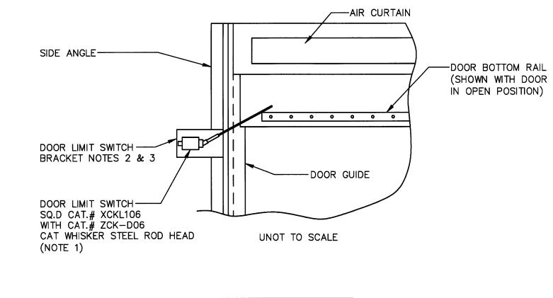
**UDOOR LIMIT SWITCH WIRING**
