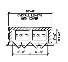
NOTE: "BIN WITH CASTERS" IS MANUALLY REMOVED FROM ENCLOSURE AND ROLLED INTO POSITION FOR TRUCK ACCESS. A LEVEL CONCERTE SURFACE AND APPROPRIATE CLEARANCES ARE TO BE PROVIDED TO PERMIT MANUAL MANEUVERABILITY.
