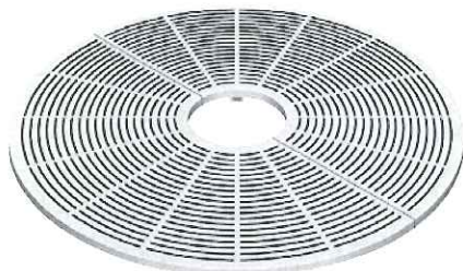
R-8876 • 72" Round 16" diameter expandable tree opening. Available with cast 18" diameter tree opening. .25" slot openings. 622 pounds per set. (Available with light openings, order as R-8876-1. 606 pounds per set.)
