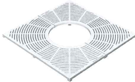
R-8704-A • 36" x 36" 16" diameter expandable tree opening. .25" slot openings. 115 pounds per set. Available with corner light openings. 9.5" x 1" grate or 7.875" x .75" lid. R-8704-A LA Order as R-8704-A LA for Los Angeles approved grate.
