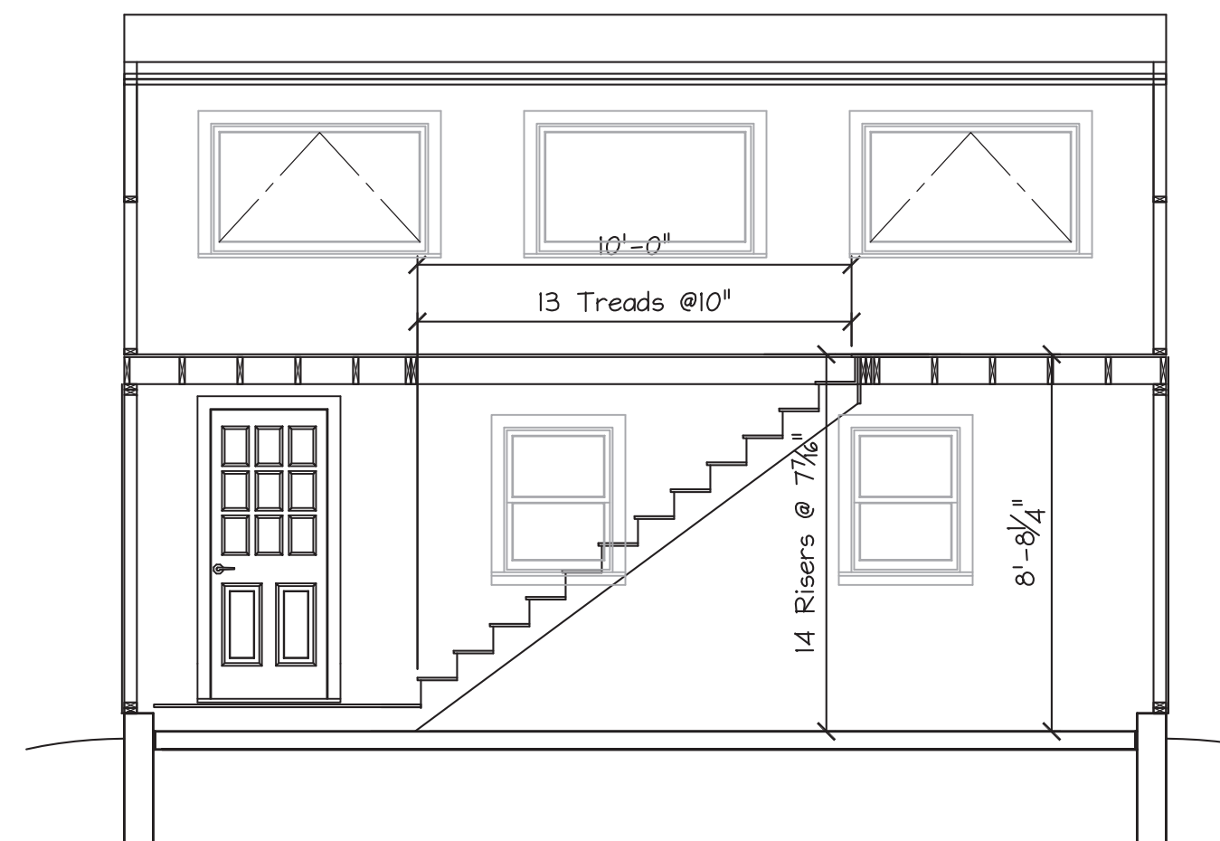
NEW CONDITION SECTION scale: 1/4" = 1'
