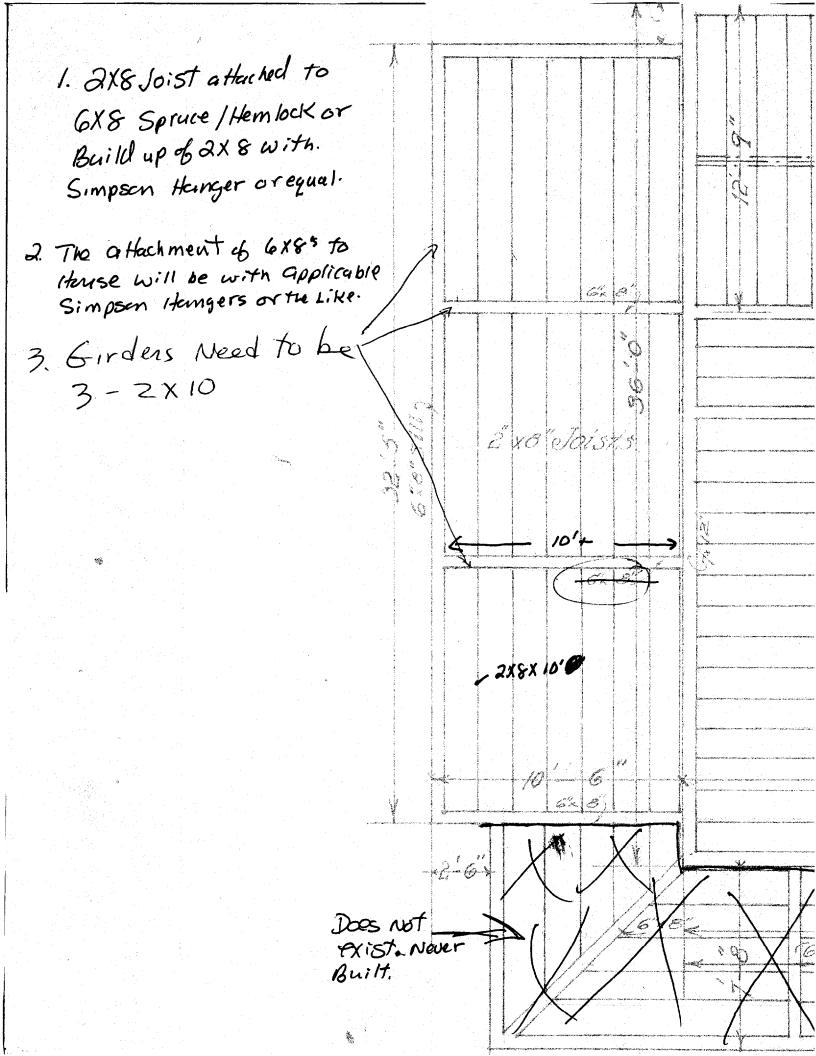
1. Roof Francis A. Joists 2x6 2-2×6 B. Plates 6x8 Sprue/ Hemlock + Dressed or 2 x 8's Builtup- + Supported By 10" Columns. C. Hipped Frame Doubled 216'5 D. Cleiling will also Be Constructed W/2x6 & Finished Phywoop panels. Panels will Be trimed Apox Size of panel 12" x 10" E. Simpson hangers 0 F. Using existing Rim soist Dista trusses
