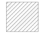
AREA OF DEMOLITION WORK TO INCLUDE REMOVALS OF WALLS, DOORS, FLOORING, CEILINGS, ELECTRICAL FIXTURES AND SWITCHES, PLUMBING FIXTURES AND PIPING. ALL ELECTRICAL CIRCUITS AND PLUMBING LINES ARE TO BE TEMPORARILY TERMINATED AND CAPPED FOR RE-USE.
