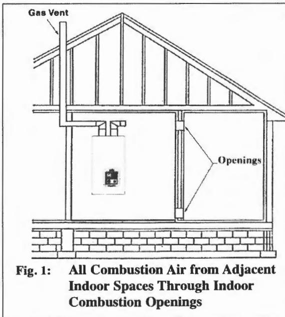
**Fig. 1: All Combustion Air from Adjacent Indoor Spaces Through Indoor Combustion Openings**
