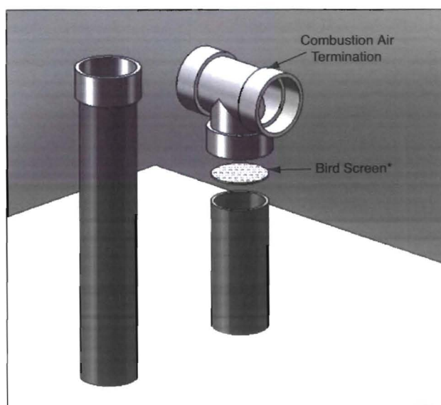
Fig. 6: Vertical Combustion Air Bird Screen Installation with Tee Termination
