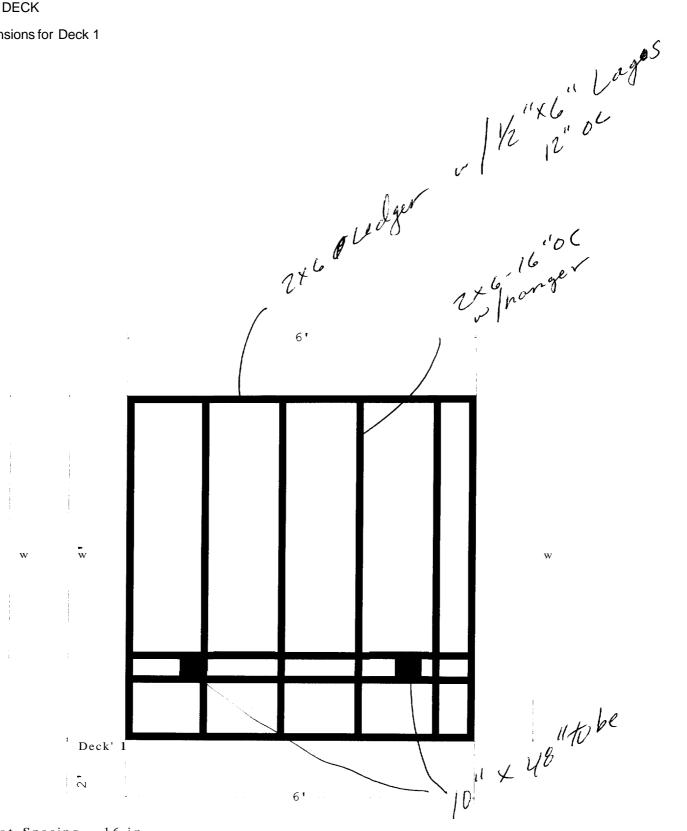
Joist Spacing = 16 in. o.c. Baluster Spacing = 3 3/4" Toe Spacing = 3 3/4" Railing Height = 36"
