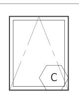
UNIT: FS M04 2004 STYLE: DECK-MOUNT FIXED SKYLIGHT MANUF: VELUX DESCRIPTION: UNIT WIDTH: 2'-6 \( \frac{9}{16} \)" UNIT HEIGHT: 3'-8 3/8" EGRESS: NO U-FACTOR: 0.43 SHGC: 0.23 VLT: 0.52
