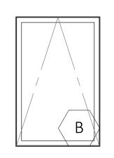
UNIT: VS M06 2004 STYLE: DECK-MOUNT VENTING SKYLIGHT MANUF: VELUX DESCRIPTION: UNIT WIDTH: 2'-6 \%\_6" UNIT HEIGHT: 3'-10 1/4" EGRESS: NO U-FACTOR: 0.43 SHGC: 0.23 VLT: 0.52
