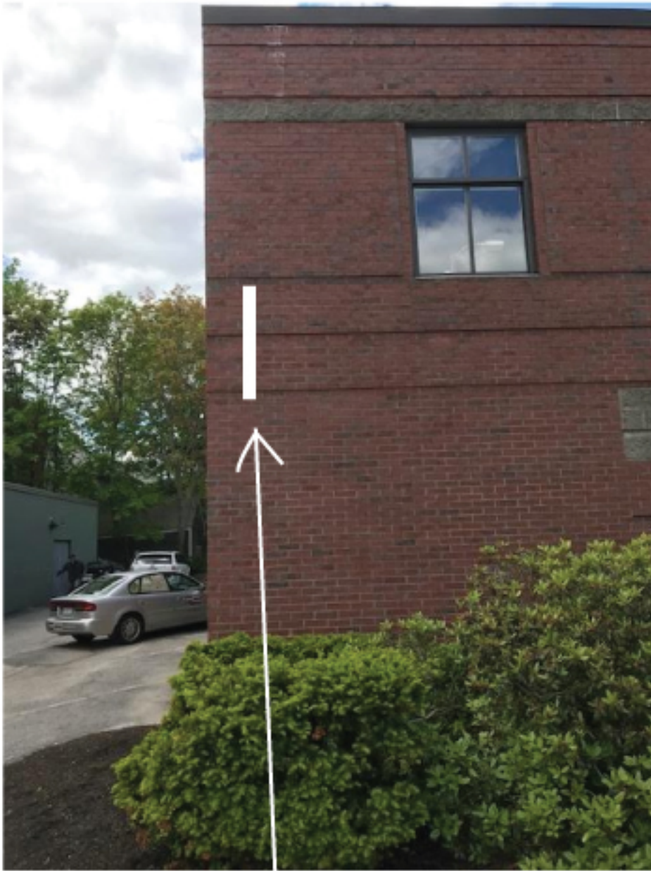
sign placement - 10' from bottom of sign to the ground
