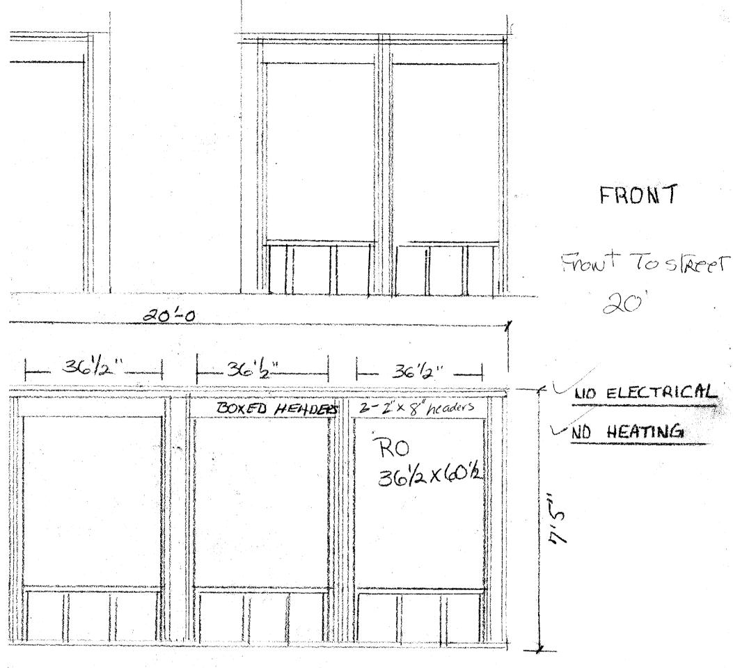
ESTERN FRAMING 2X6 CONST 16 oc ATHING - VINYL SIDING PEA - 6/1 LOW E NAILING FINS
