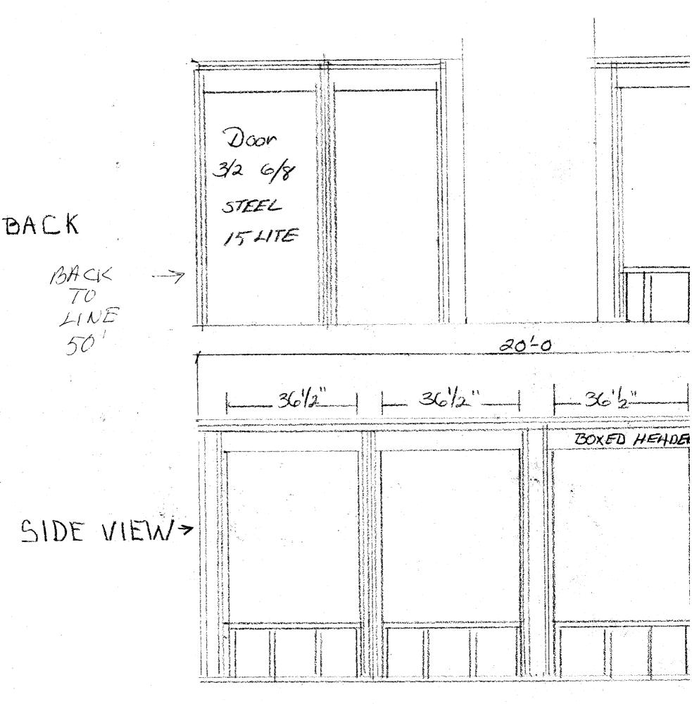
STANDARD WESTERN FRAMING 2X6 CON ZIG OSB SHEATHING - VINYL SIBING DH WINDOWS TEA - 6/1 LOW E NAILI EXTERIOR DOOR IS LITE STEEL ALUMINUM FLASHING
