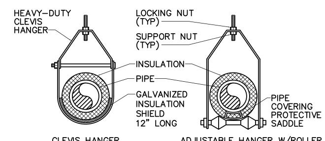
CLEVIS HANGER ADJUSTABLE HANGER W/ROLLER (FOR PIPES 2-1/2" & SMALLER) (FOR PIPE 3" THROUGH 6")
