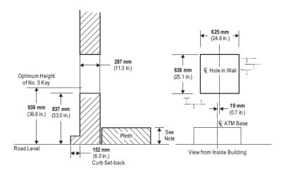
**Note:** For UL security enclosures, this dimension is **271 mm** (10.7 in.). For CEN security enclosures, this dimension is **262 mm** (10.3 in.).
