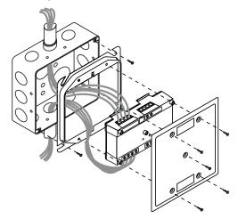
**SIGA-MCC1** and **SIGA-MCC2**: mount the UIO motherboard inside a suitable EDWARDS enclosure with screws and washers provided. Plug the SIGA-MCC1 or SIGA-MCC2 into any available position on the motherboard and secure the module to the motherboard with the captive screws. Wiring connections are made to the terminals on the motherboard (see wiring diagram). UIO motherboard terminals are suited for #12 to #18 AWG (2.5 mm² to
