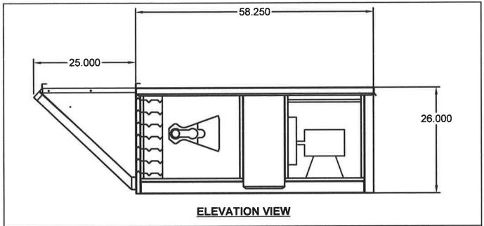
\*Standard configuration for unit access is on the right-hand side, when looking into the unit intake in the direction of airflow.
