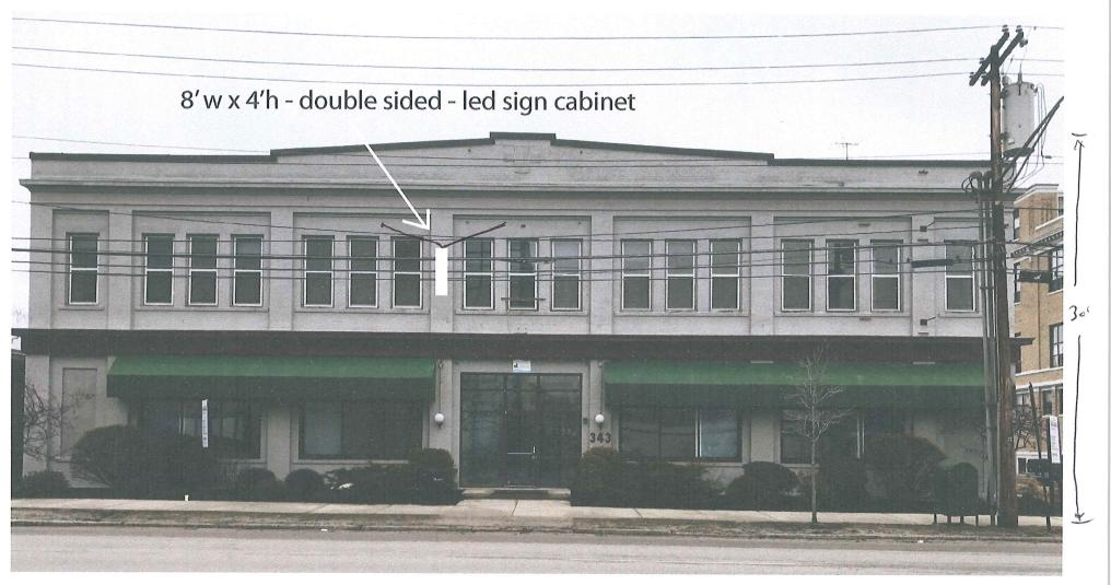
sign bottom will be 17' from the ground mounted to the building with steel brackets - which are through bolted into the building and guide wires on the top of the sign attached to the building.
