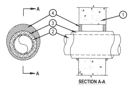
Wall Assembly — Min 3-3/4 in. (95 mm) and 5 in. (127 mm) thick reinforced lightweight or normal weight (100-150 pcf or 1600-2400 kg/m³) concrete required for F and FH Ratings of 1 and 2 Hr, respectively. Wall may also be constructed of any UL Classified Concrete Blocks\*. Max diam of opening is 7-1/2 in. (191 mm).
