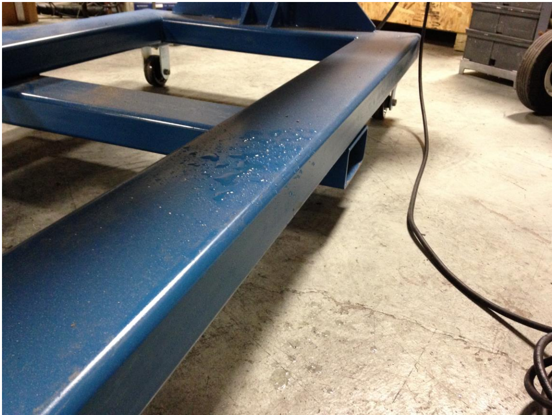
Roll-over – Post-Test (Battery Stack Leak)
