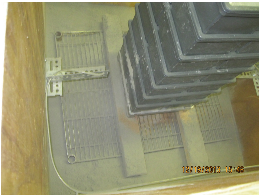
Photo 2 – File No. RC13-0692 Dust test setup during dust testing
