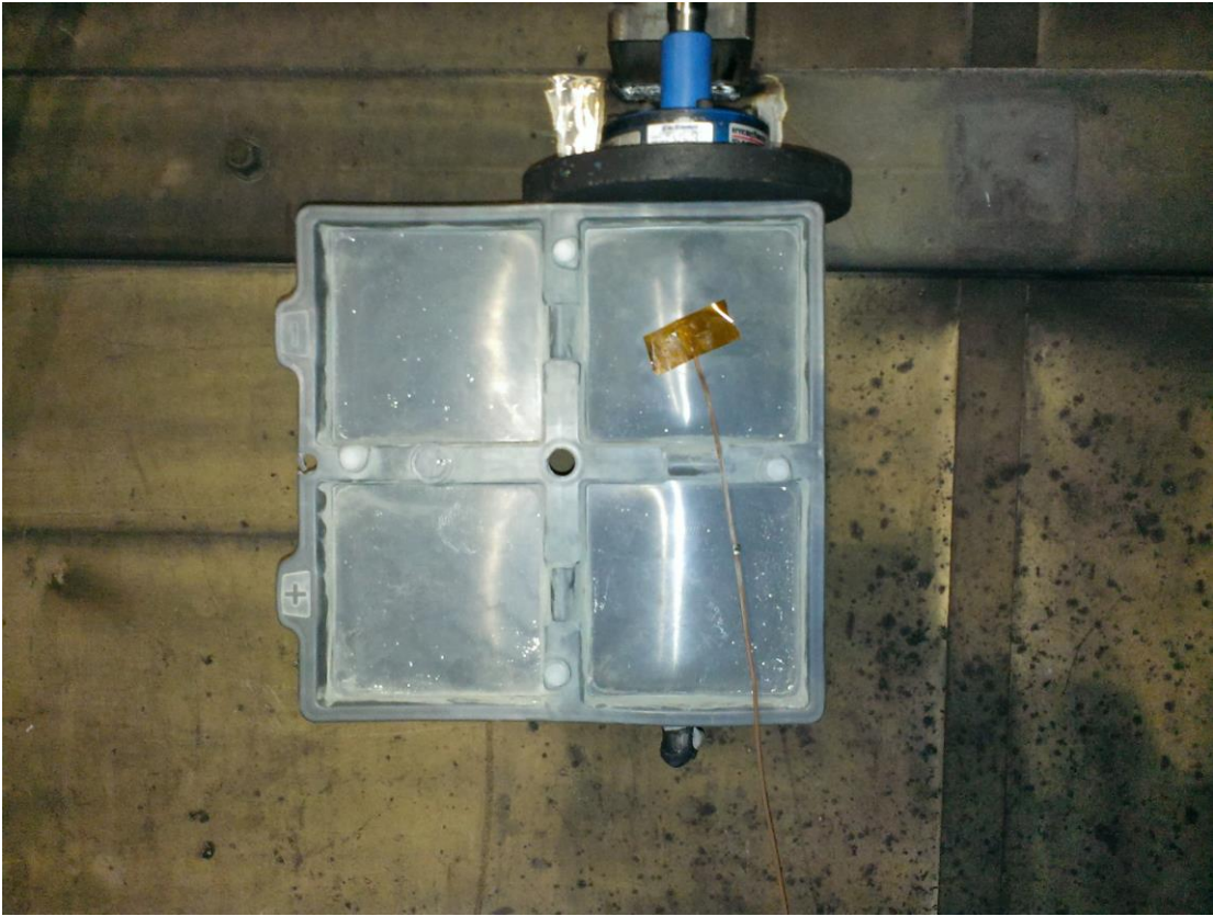
Nail Penetration – Post-Test (Cell)
