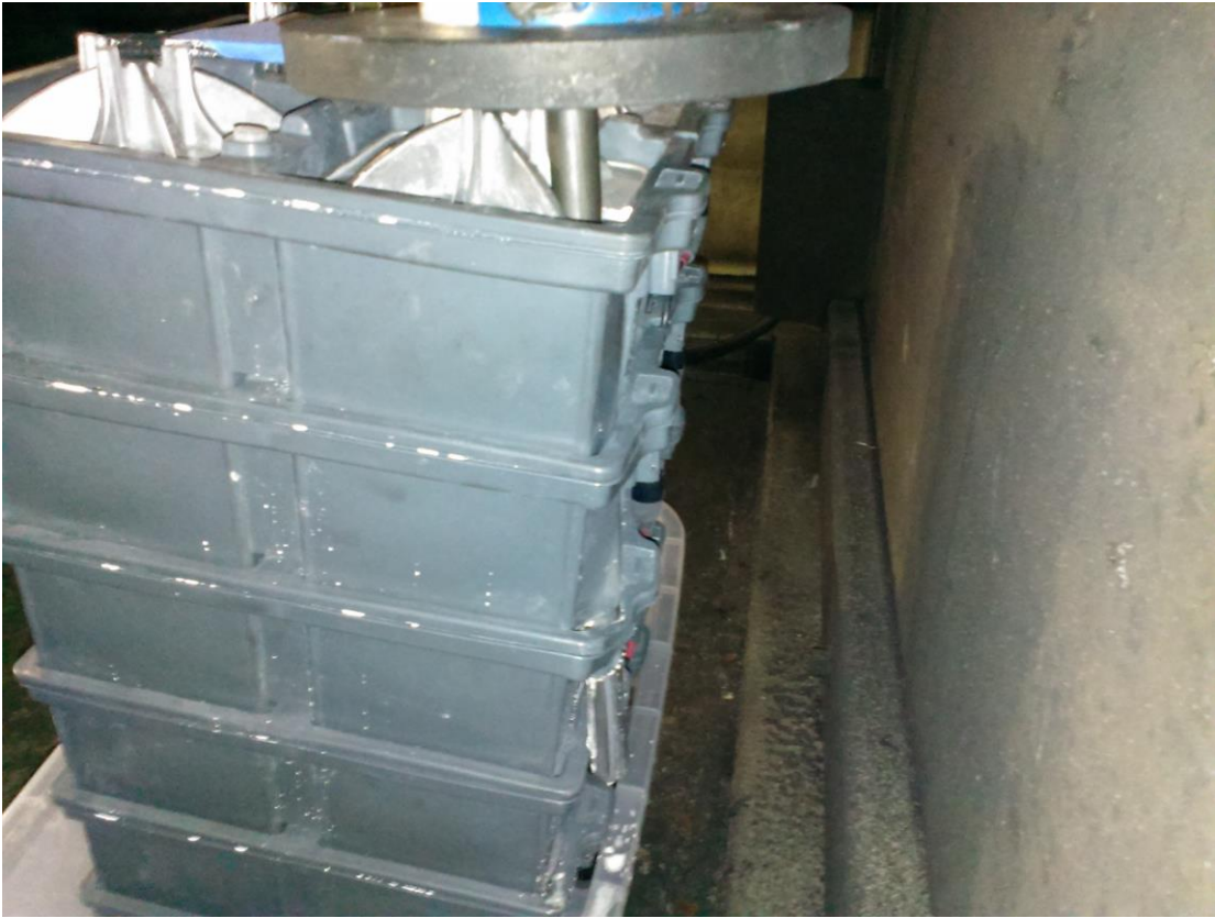
Nail Penetration – Post-Test (Battery Stack)
