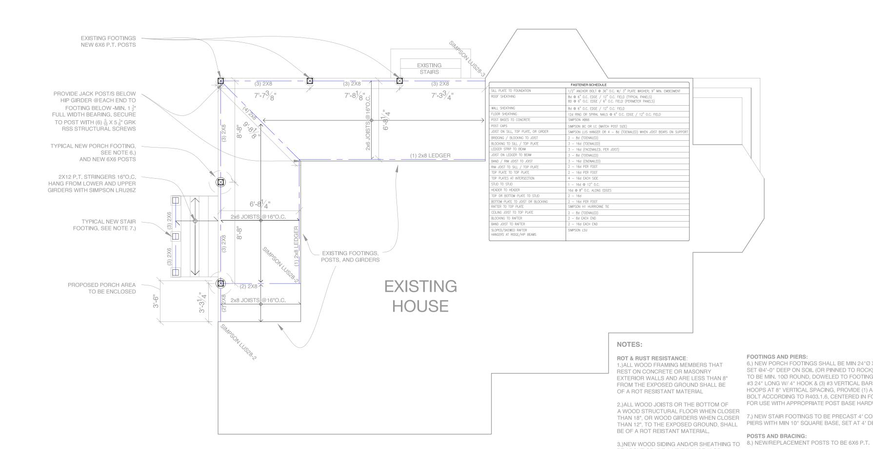
6.) NEW PORCH FOOTINGS SHALL BE MIN 24"Ø X 8" SET @4'-0" DEEP ON SOIL (OR PINNED TO ROCK). PIERS TO BE MIN. 10Ø ROUND, DOWELED TO FOOTING WITH (2) #3 24" LONG W/ 4" HOOK & (3) #3 VERTICAL BARS & #3 HOOPS AT 8" VERTICAL SPACING, PROVIDE (1) ANCHOR BOLT ACCORDING TO R403.1.6, CENTERED IN FOOTING, FOR USE WITH APPROPRIATE POST BASE HARDWARE
