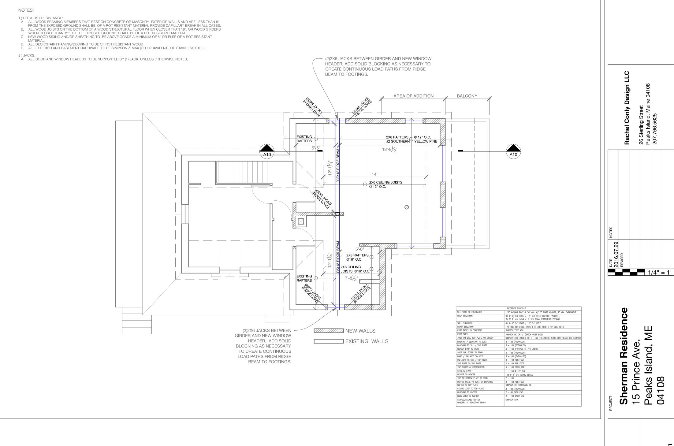
Proposed Roof Framing Plan
