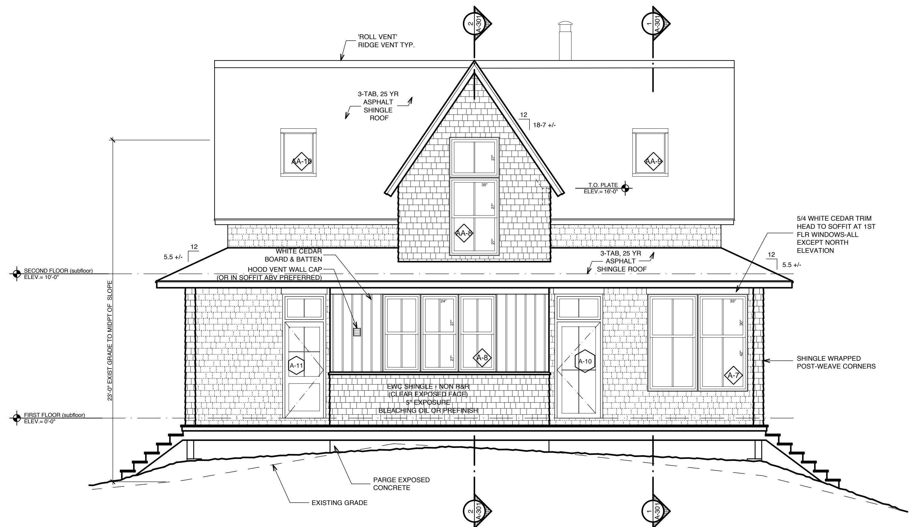
4 SOUTH ELEVATION SCALE: 1/4" = 1'-0"
