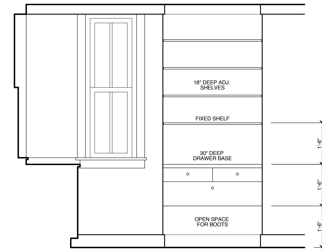
3 KITCHEN ELEVATION - West Wall SCALE: 1/2" = 1'-0"
