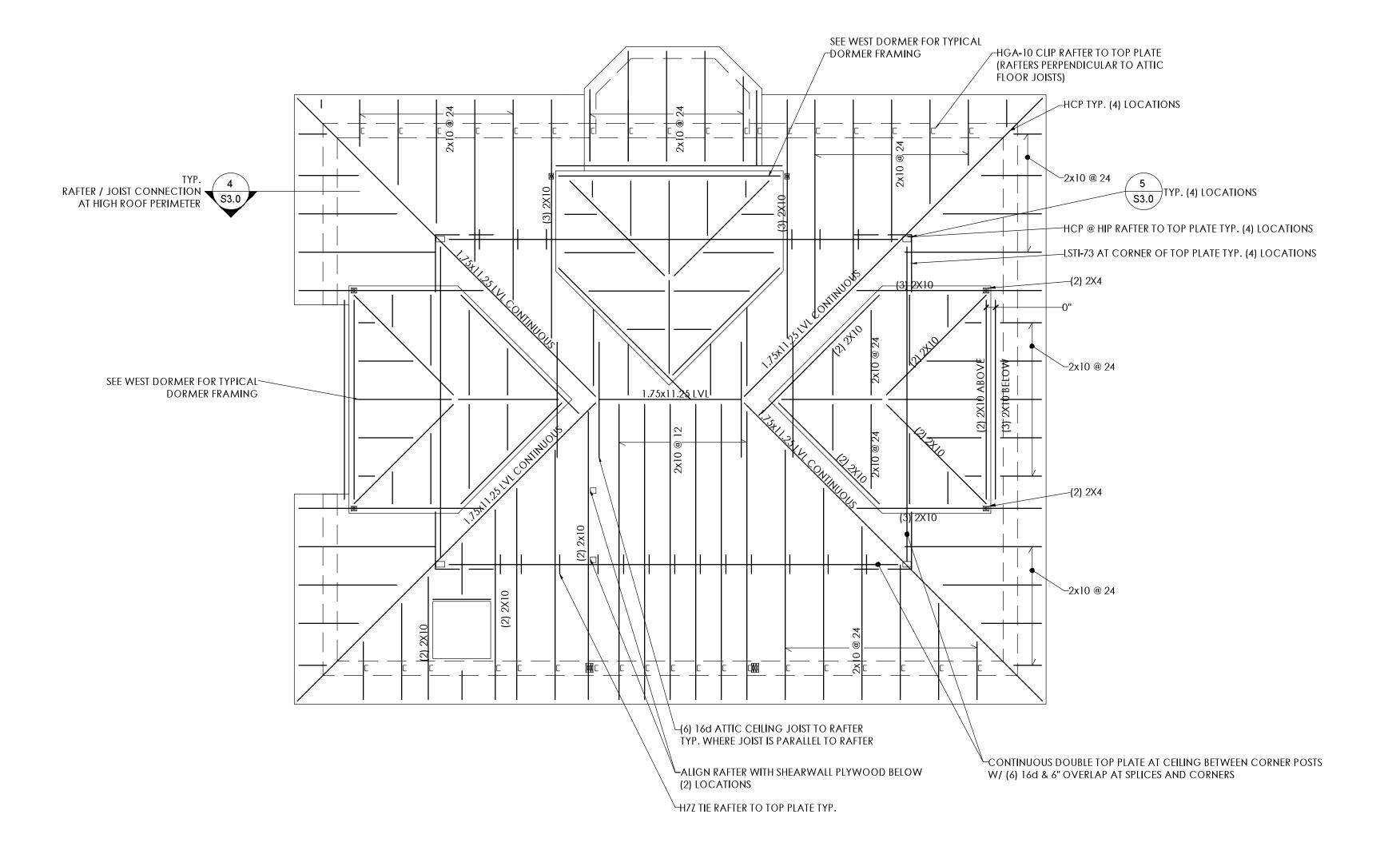
NOTE: ALL FRAMING NOT LABELED TO BE 2x10, TYP. ALL POSTS NOT LABELED TO BE (2) 2X4 OR (2) 2X6 (MATCH WALL STUD DEPTH)
