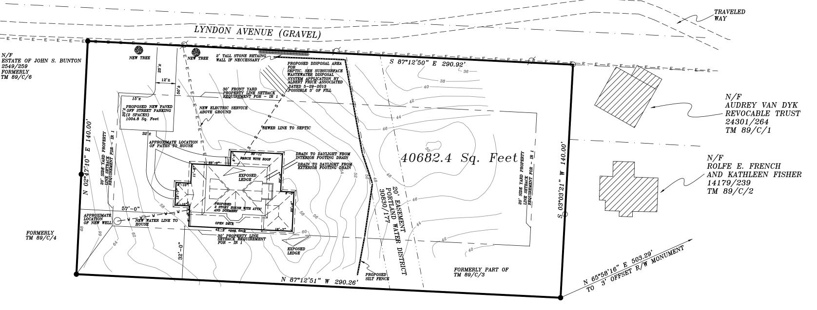
N/F BUNTON 30443/294 FORMERLY TM 89/D/8 AREA OF LOT = 40682.4 Sq. Feet AREA OF LOT TO BE COVERED BY STRUCTURE= 2,255 SF PERCENTAGE OF LOT COVERAGE = 5.54 PERCENT PROPOSED FINISH FLOOR ELEVATION = 61' SOIL TYPE IS HsC
