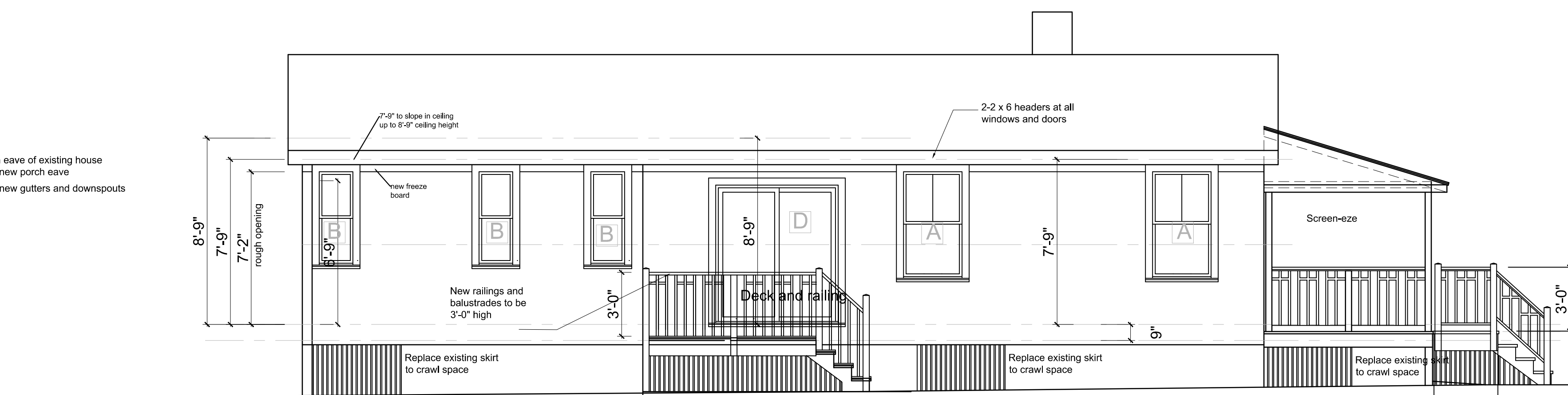
SOUTH ELEVATION AND SIDE PORCH
