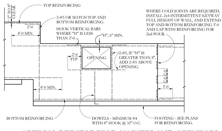
TYPICAL REINFORCING AT STEPS AND OPENINGS
