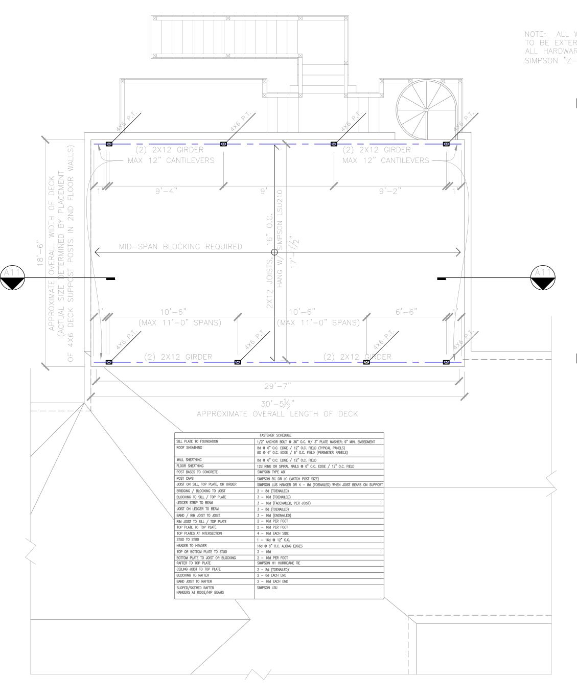
NOTE: ALL WOOD (AND WOOD COMPOSITE) FRAMING & FINISH MATERIALS TO BE EXTERIOR RATED AND ROT RESISTANT.
