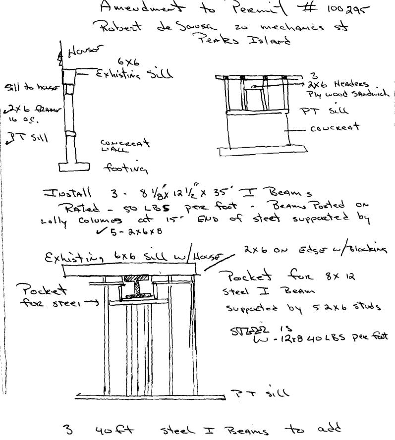
3 40 ft steel I Beams to add As CARRING BEAMS - supposet Exhisting floor Joist Lolly columns as needed Corcreat
