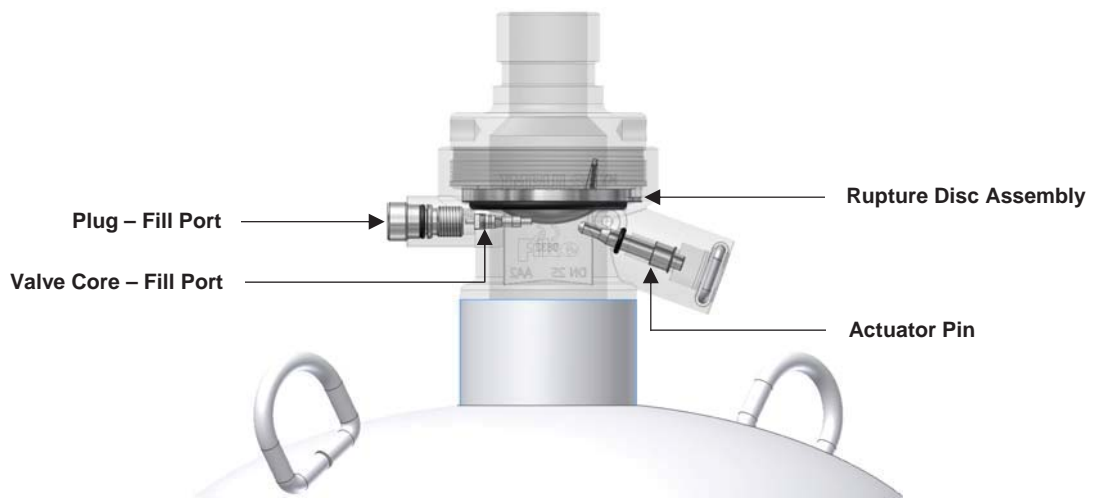
Internal View – 1” Impulse Valve
