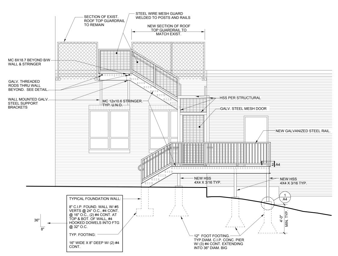
3 STAIR 4 - New Work Elevation
