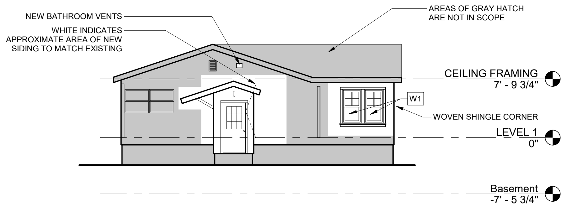
4 Exterior Elevation - West - New Construction 1/8" = 1'-0"
