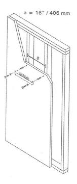
Install mounting bracket and CombiPLUS on metal studs as per illustration. Drill 5%" pilot holes to insert anchors. Ensure that holes are located in the center of each metal stud. Use appropriate fasteners to mount CombiPLUS to metal studs (not supplied). Secure with bolts to metal studs as shown.
