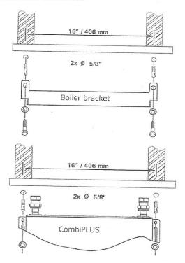
Install mounting bracket and CombiPLUS on wood studs as per illustration. Drill <sup>3</sup>/<sub>16</sub>" pilot holes to insert mounting bolts. Ensure that holes are located in the center of each wood stud. Secure with bolts to wooden studs as shown.
