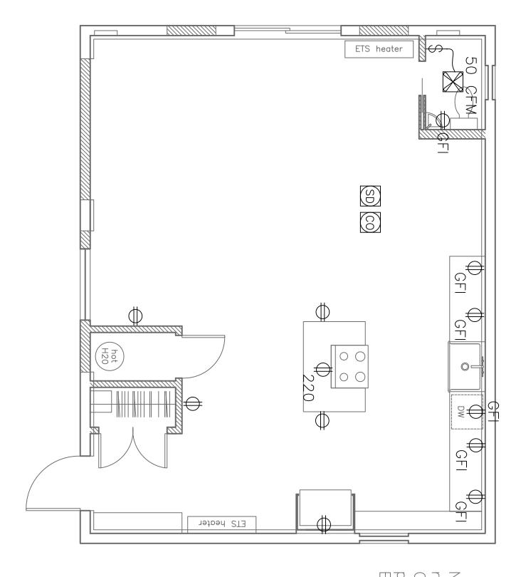
Notes: Lighting plan is responsibility of Electrician. Outlet quantity and placement at discretion of Electrician— to code
