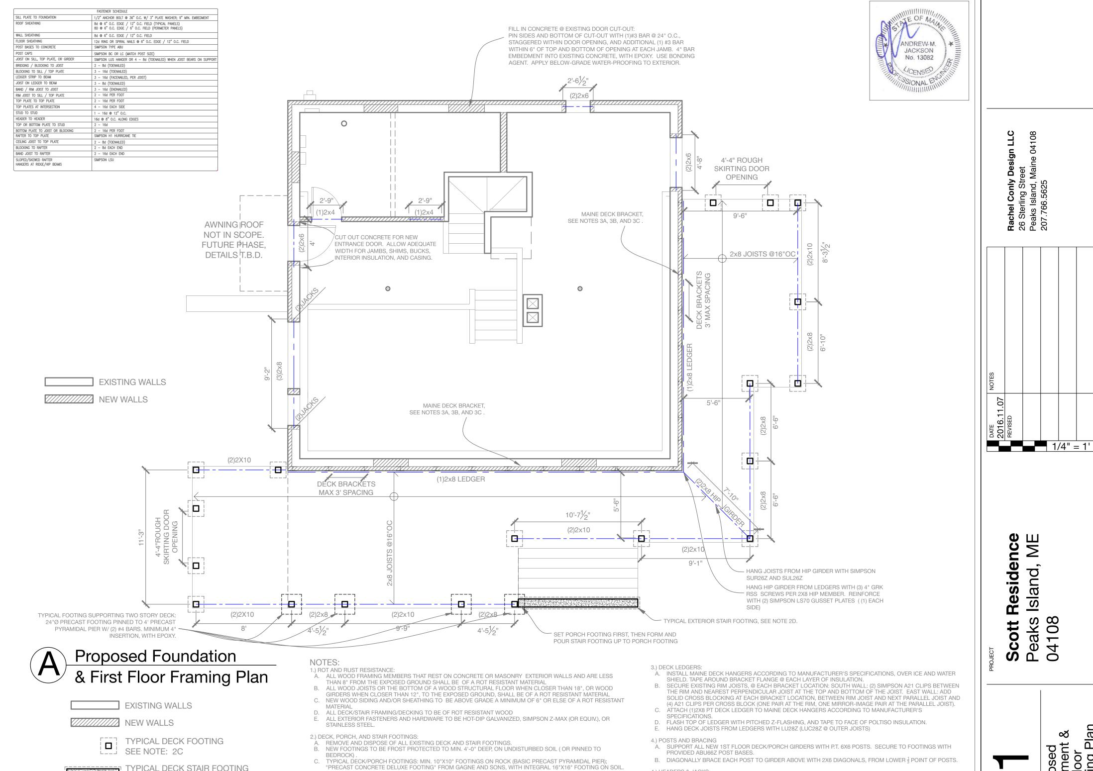
SECURE ABU66Z POST BASE TO CAST-IN-PLACE THREADED INSERT @ EACH FOOTING WITH  $\frac{1}{2}$ " THREADED ROD,
