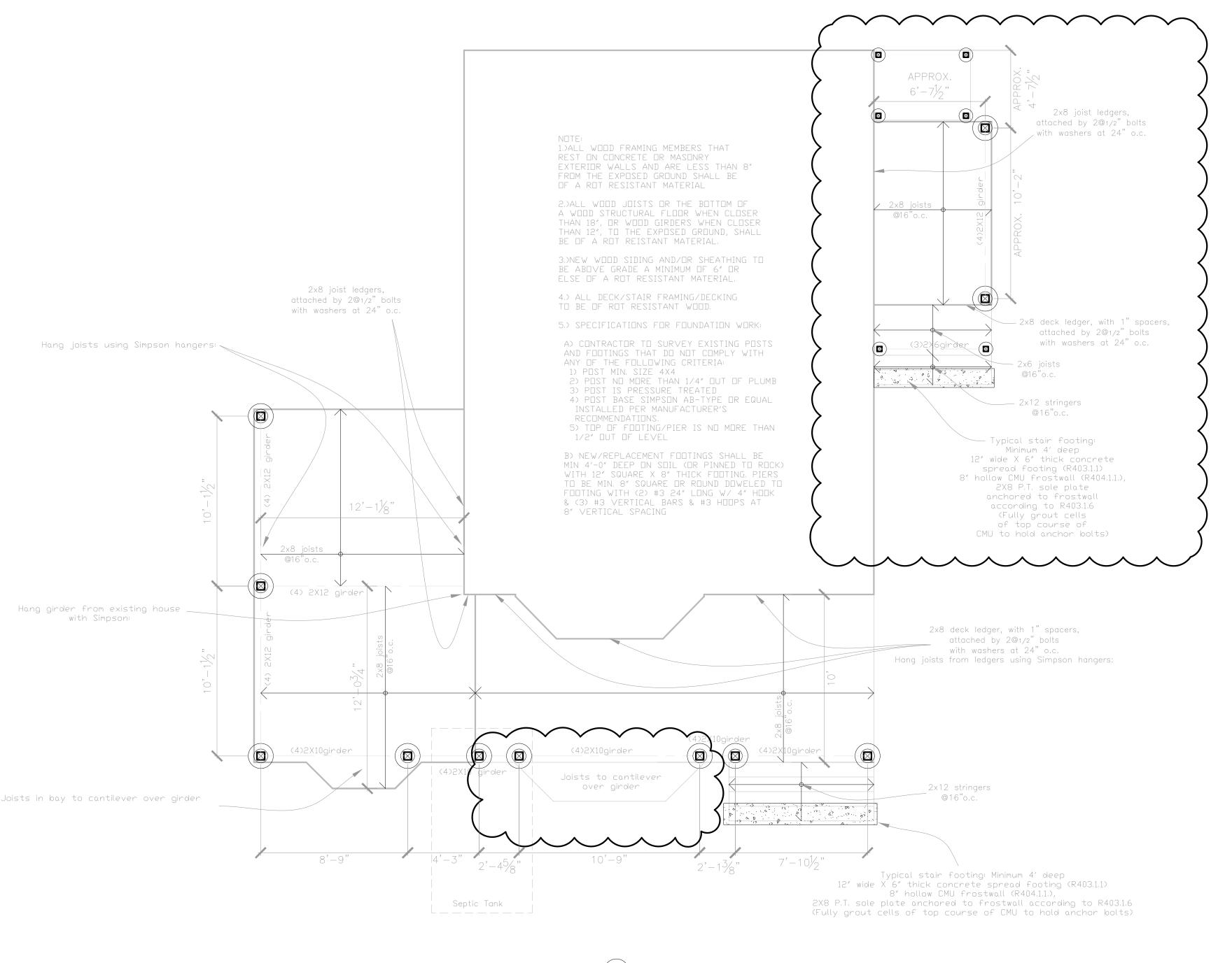
typical footing: 6X6 pressure treated post 10"Ø sonotube on 24"Ø footing, min. 4' below grade
