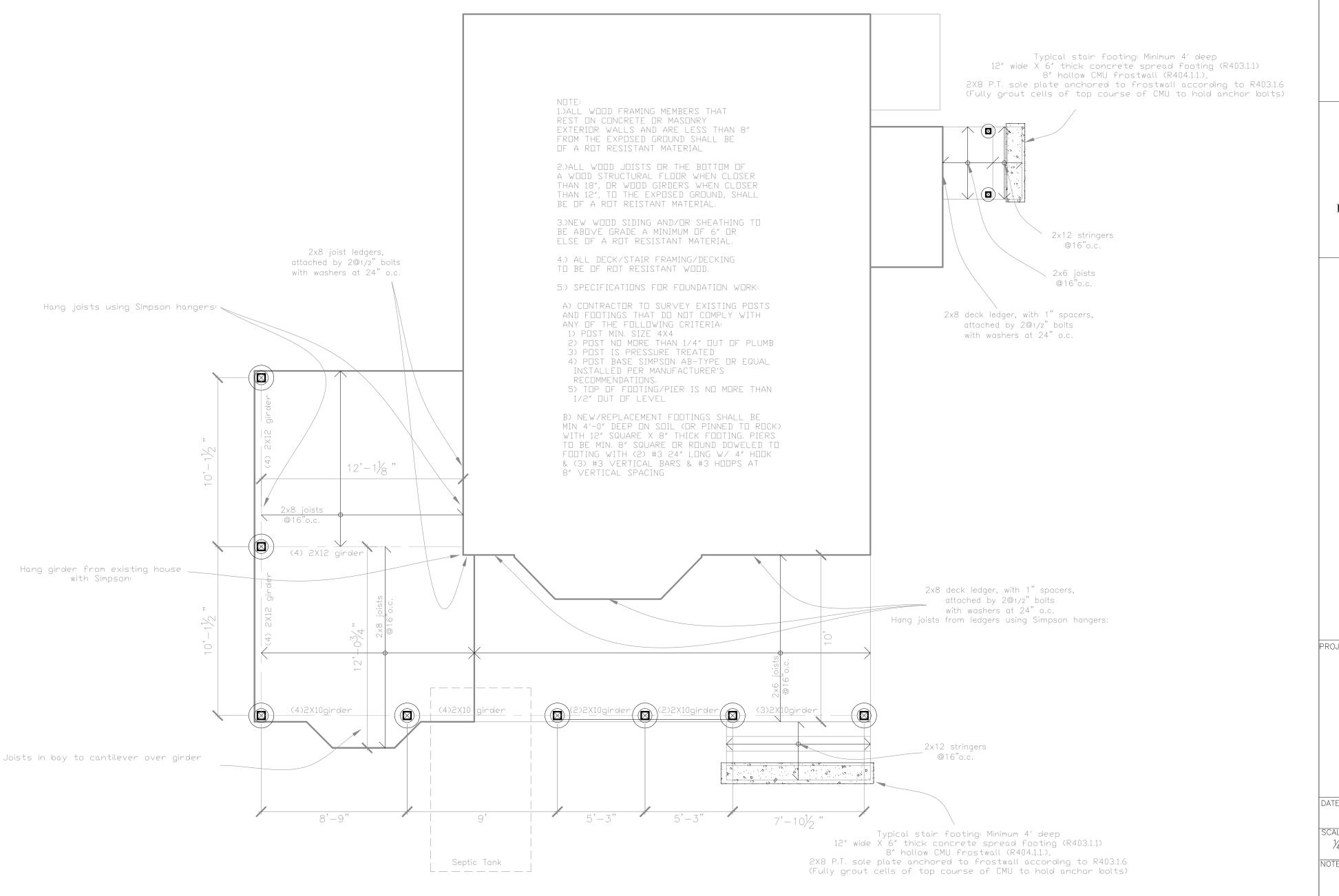
typical footing: 6X6 pressure treated post 10"ø sonotube on 24"ø footing, min. 4' below grade
