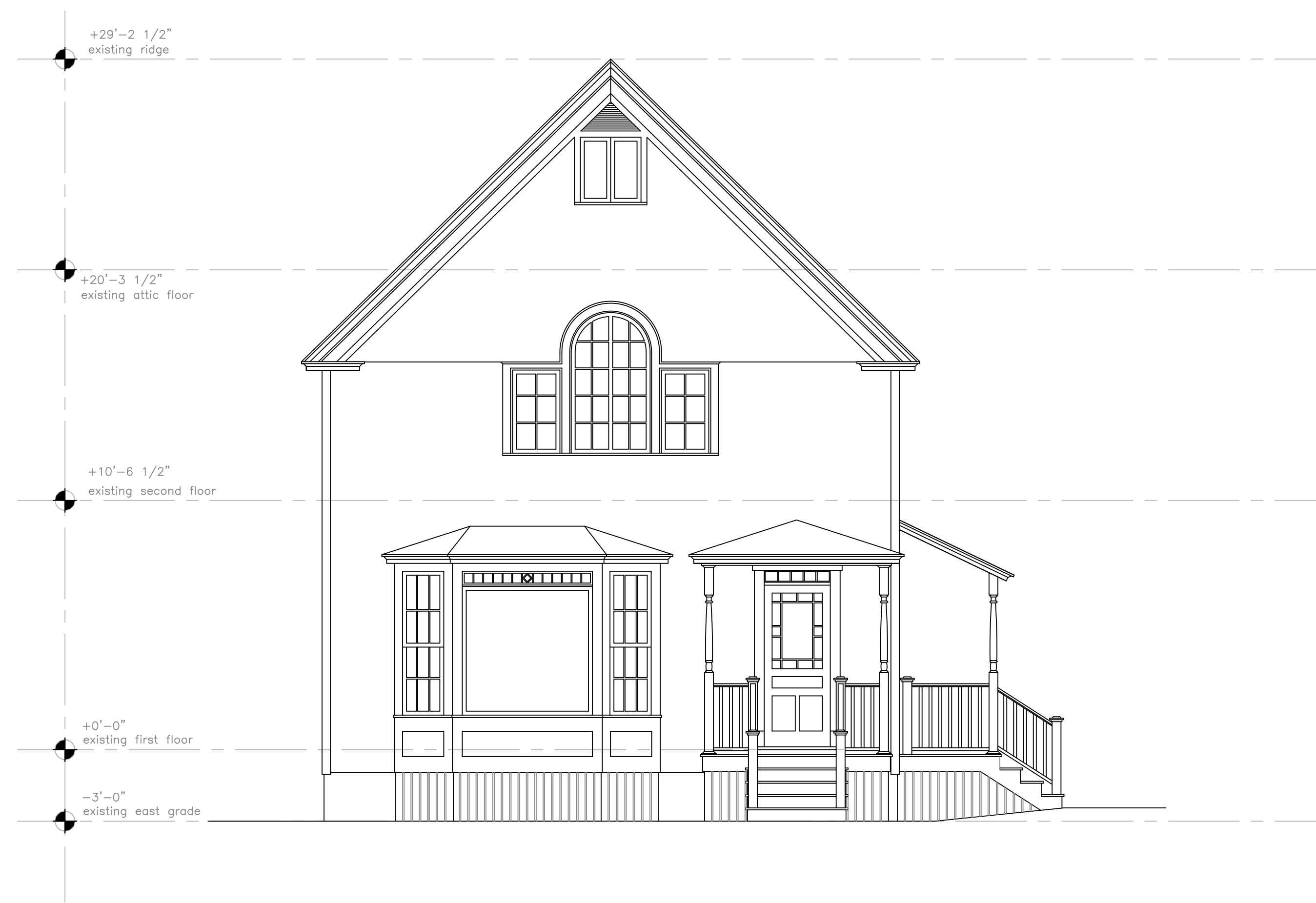
(A) Existing South Elevation 1/4" = 1'-0"
