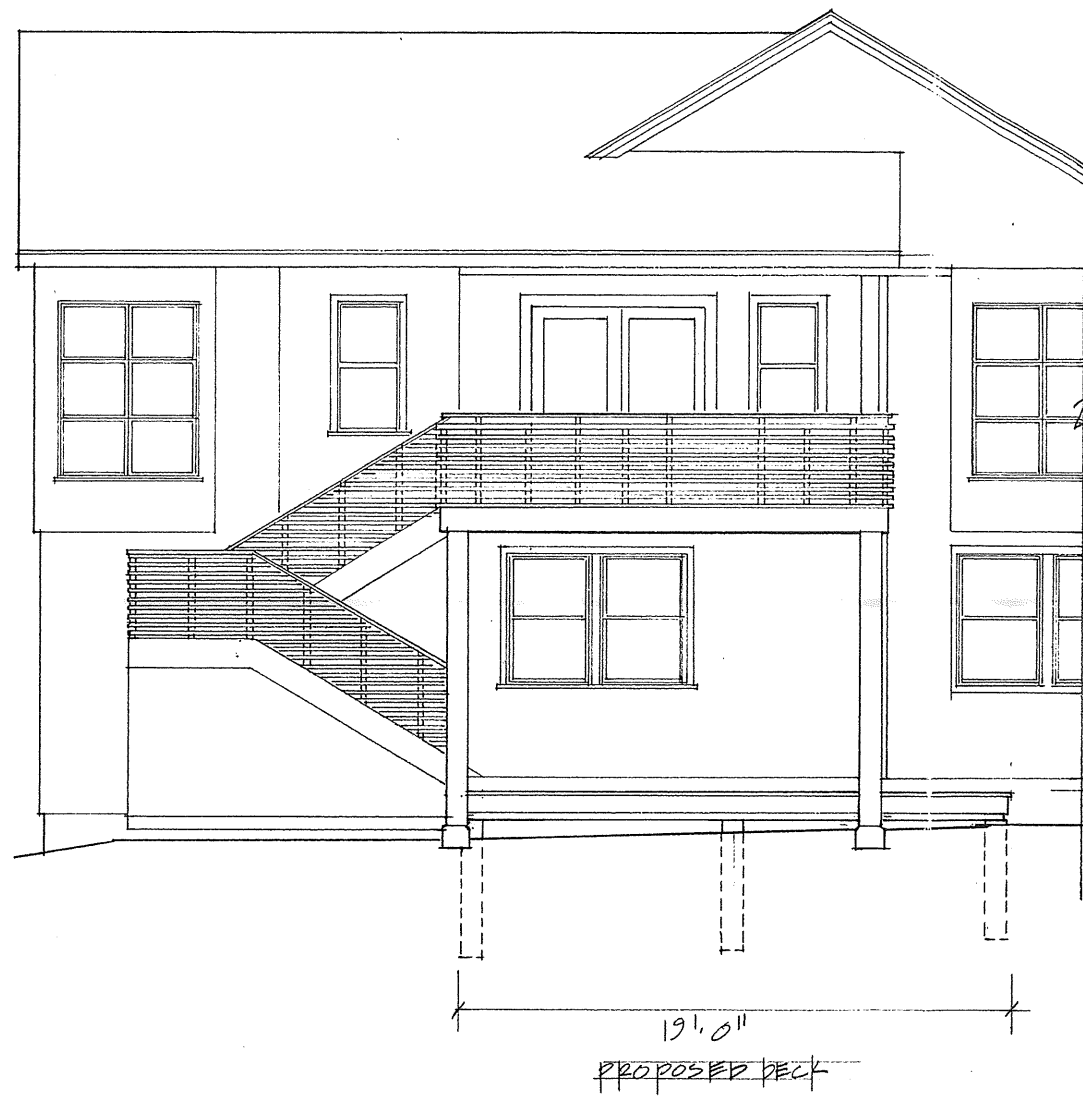
(A) APPENDUM FOR DECK @ GRADE: SOUTH ELEVATION 1/4" = 1'-0"
